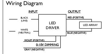
Input, Output and 0-10V Dimming use lead-wires.
